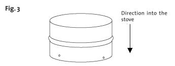
The adaptor should be inserted into the stove until the bead on the adapter is flush with the top, back or side casting. Now the adaptor is ready to accept single or double walled stove pipe. See **figure 4**.
